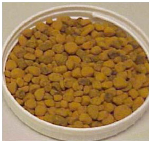
Iron oxide coated sand Source: UNESCO-IHE
