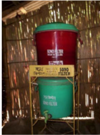
An Alcan filter (left) under testing in Azimpur village, Manikgonj district, Bangladesh, and a Sono arsenic removal filter (right) (Source: IRC)
