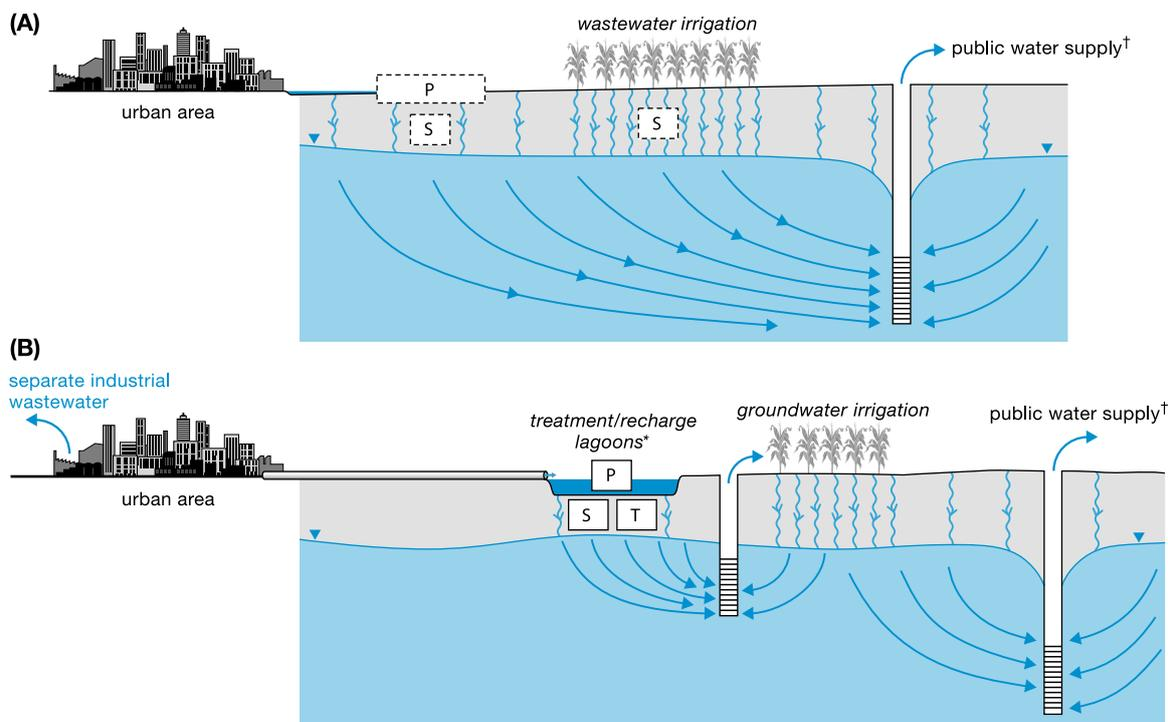
P/S/T    P/S/T    effective level of wastewater treatment (P= primary; S = secondary; T = tertiary)
