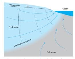
Figure 2. Fresh – salt water interface of an unconfined aquifer (illustration after Fitts, 2002)
