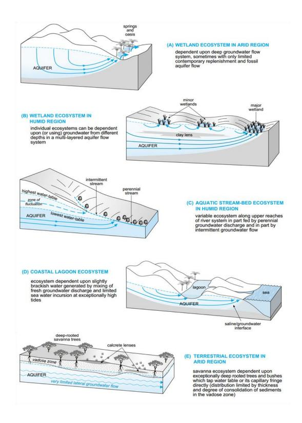
Figure 3. Main classes of groundwater related ecosystems and their associated groundwater flow regime (GW-MATE, 2006)
