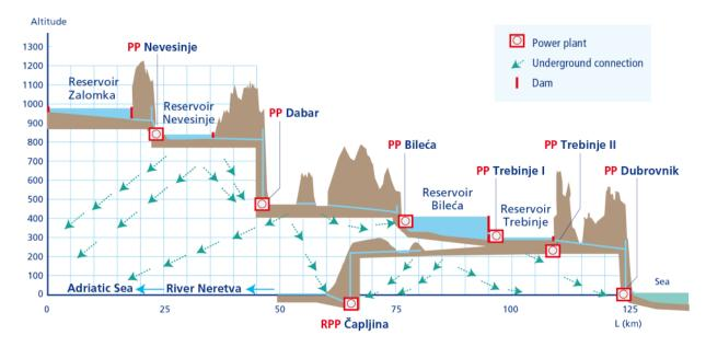
Longitudinal profile of Trebišnjica Hydrosystem, with directions of groundwater flow
