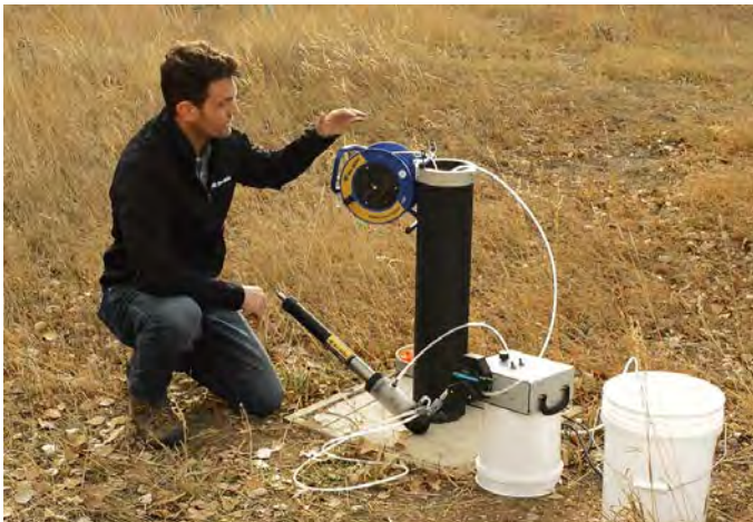
Figure 15.8 Left : Low-flow sampling equipment. Courtesy of In-Situ ( https://in-situ.com/us/low-flow-sampling ). Right : Low-flow sampling at a site in Pennsylvania, United States. Photo courtesy of Jeff Manuszak.
