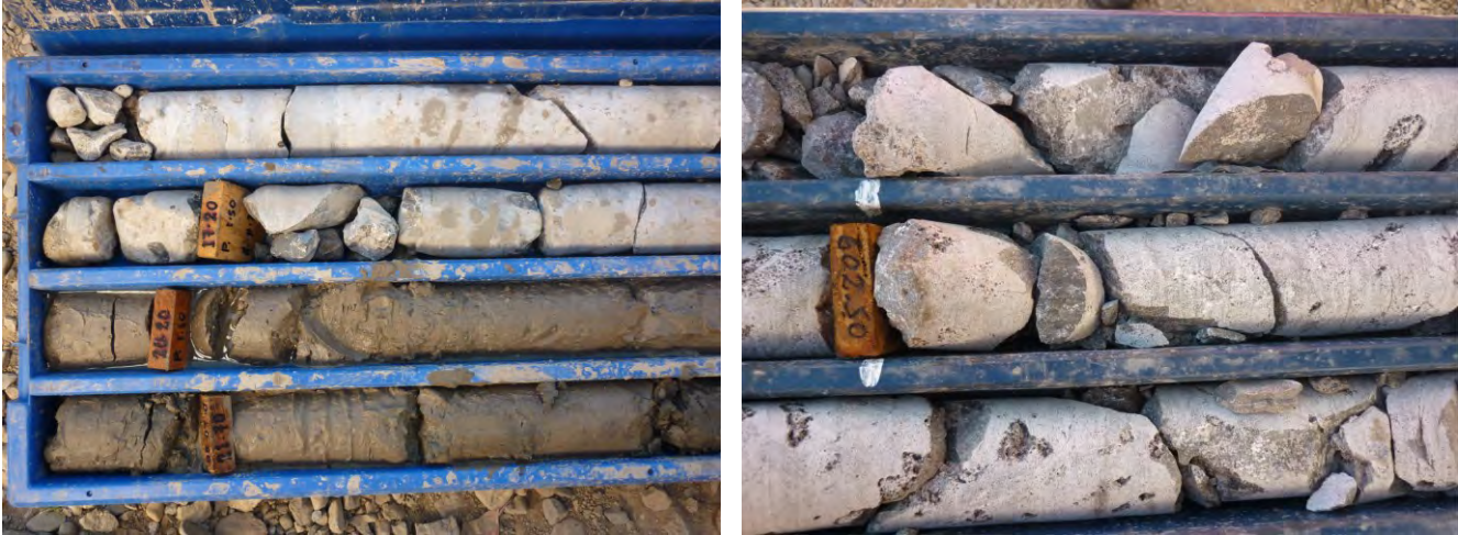
Figure 14.16 Dolomitic rock core from an exploration boring at a site in Peruvian Andes. Left: Upper, highly weathered portion of bedrock with a clay-filled cavity. Right: Broken-up core in highly fractured and karstified (vuggy) section of bedrock at ~600 meters (1,970 feet) below ground surface.
