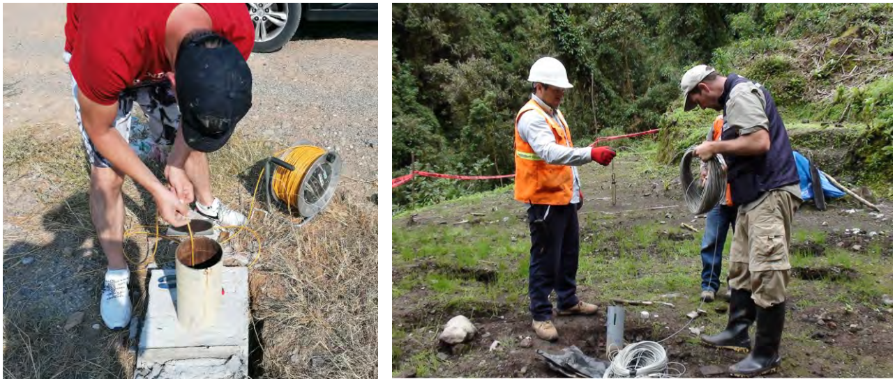
Figure 15.3 Examples of manual water-level measurements in monitoring wells. Left : Student of hydrogeology learns how to take measurement with an acoustic sounding probe. Courtesy of Zoran Stevanović. Right : Taking measurement at a 385-m deep monitoring well in Peruvian Andes with an electronic sensor probe.
