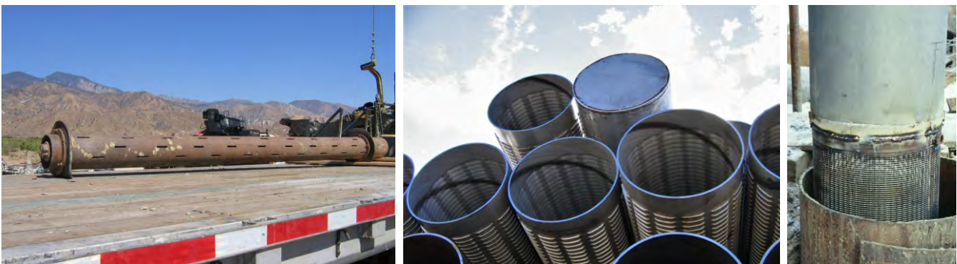
Figure 16.20 Common types of screens for high-capacity production wells. Left : Slotted casing, photo courtesy of Adrian Ezeagy. Middle : Shutter type screen, photo courtesy of Adrian Ezeagy. Right : Continuous slot wire-wound stainless-steel screen (often referred to as Johnson screen) welded to the riser pipe and being lowered into a newly drilled well.
