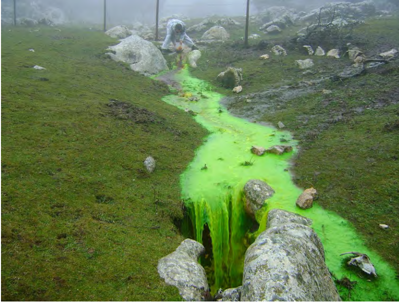
Figure 5.34 Dye tracing test with uranine in the karst system of Alta Cadena range near Malaga, Spain. Courtesy of Bartolome Andre Navarro, CEHIUMA.
