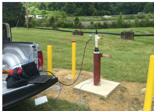
Figure 15.16 Left : Hydrogeologist Bob Seymour holds a solid cylinder (“slug”) soon to be inserted into a monitoring well as part of slug testing at the Atlantic Steel brownfields site in Atlanta, Georgia. Right : Setup for an air-pressurized slug test. Photo courtesy of Dawit Yifru.
