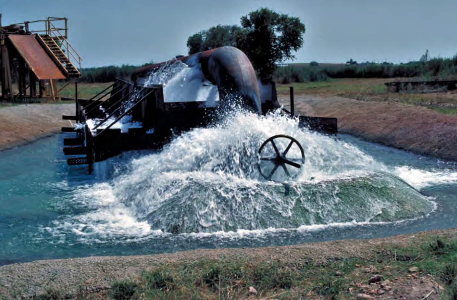
Figure 7.28 The highest capacity drilled well in the world, capable of sustained pumping of 40000 gallons per minute ( 2.5 \text{ m}^3/\text{sec} ), located on the Ron Pucek's Catfish Farm near San Antonio, Texas. Photo copyright by Gregg Eckhardt; printed with kind permission.
