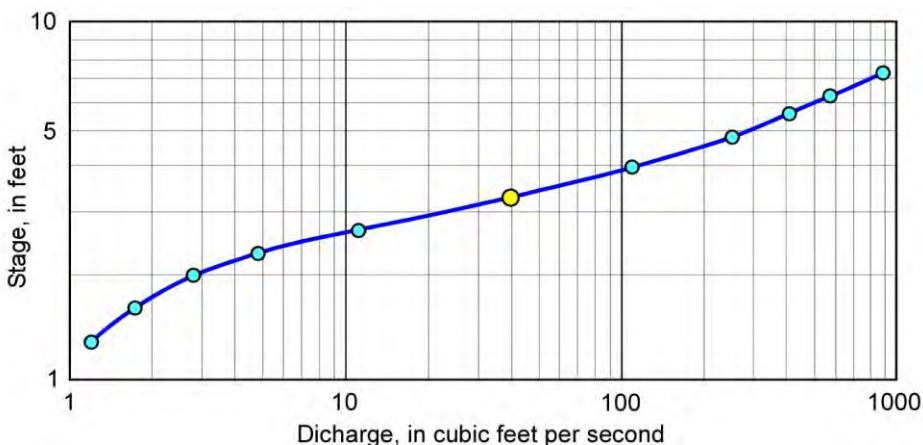
Figure 15.14 Example of a typical stage–discharge relation; here, for the large yellow dot, the discharge of the stream is 40 cubic feet per second ( \text{ft}^3/\text{s} ) when the stage is 3.30 feet (ft). The smaller blue dots on the curve represent concurrent measurements of stage and discharge. Modified from USGS, 2005, in public domain.
