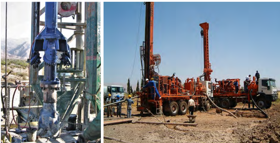
Figure 16.18 Left : Combined roller cone bit in two stages for drilling deep, large-diameter production wells. Photo courtesy of Adrian Ezeagy. Right : Drilling rigs in operation in northern Iraq (Kurdistan Province). The combined rotary and down-the-hole hammer (DTH) techniques are applied to drill formations of loose topsoil and clay, and underlying limestone. Courtesy of Zoran Stevanović.
