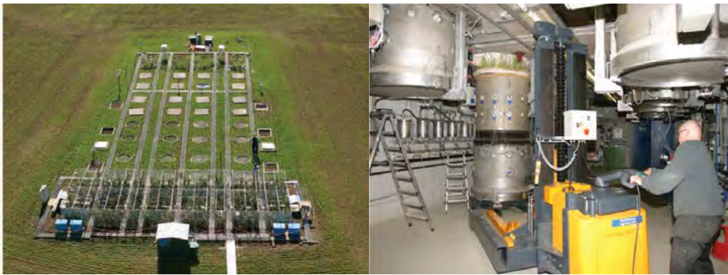
Figure 8.27 Left : Array of lysimeters operated by Helmholtz Center Munich, Germany. Right : Below-ground view of one of the lysimeters. Photographs courtesy of Dr. Sascha Reth.
