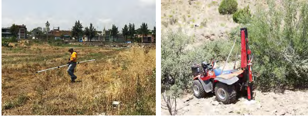
Figure 14.2 Left : Electromagnetic survey (EM) with terrain conductivity meter (antenna). Photo courtesy of Jeff Manuszak. Right : Shallow seismic reflection survey using light ATV mounted Accelerated Weight Drop in rugged terrain. Photo courtesy of Finn B. Michelsen.
