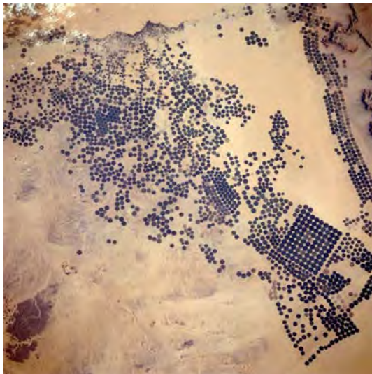
Figure 16.16 This photograph taken in 1990 by a Space Shuttle mission shows a location southwest of Riyadh in the Jabal Tuwayq area of Saudi Arabia. “The circular features that dot the desert landscape in this near-vertical photograph are created by pivoting sprinklers, a method of irrigation whereby water from a central well is spread by a sprinkler pivoting around that well. The diameter of these circular fields can vary from several hundred feet (tens of meters) to over a mile (2 kilometers)....The water is being extracted from subsurface reserves that infiltrated deep aquifers during geological periods when the climate was much wetter than at present.... The significance of the Saudi expanded irrigated agriculture is that the depletion of this finite water resource is a short-term solution to a long-term need that will still exist when the water has been extracted.” https://eol.jsc.nasa.gov/ ; in public domain.
