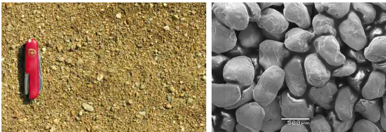
Figure 2.3 Left : photograph of coarse alluvial sand with gravel. Right : ESM (Electron Scanning Microscope) image of uniform, pure quartz sand. Photo courtesy of Dr. Scott Chumbley, Iowa State University.)
