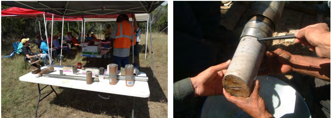
Figure 14.15 Left : Students of hydrogeology attending session on rock coring technologies, Texas Hydro-Geo Workshop, Boerne, TX, 2015. Right : Core sample of compact limestone taken by wire line technique. Courtesy of Zoran Stevanović.
