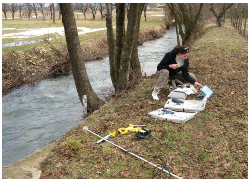
Figure 15.6 Monitoring spring water quality. Field equipment includes probes for measuring electrical conductivity, pH, water temperature, redox potential (ORP), and turbidity. Note a flow measurement device in the front. Courtesy of Zoran Stevanović.
