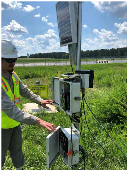
Figure 15.1 Monitoring well equipped with automatic water-level sensing and recording instruments programmed to make measurements at 15-minute intervals. The well is part of a SCADA system and has autonomous solar energy source. Courtesy of Nick McMillan.
