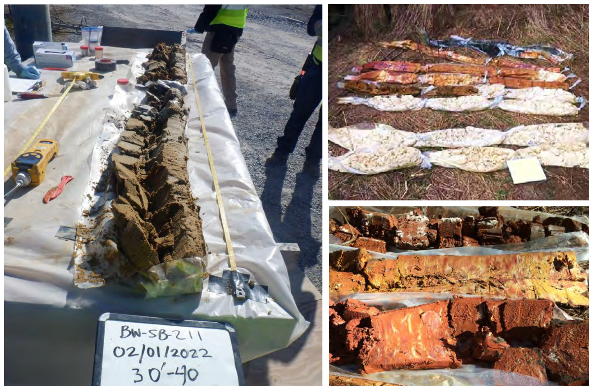
Figure 14.14 Left : Examining and sampling a 10-foot sonic core of silty sand retrieved in plastic sleeve. Courtesy of Nick McMillan. Right : Sonic cores of clay (yellow to brown color) and white “sand”. In this case, “sand” is weakly cemented Ocala limestone which lost its cohesion due to sonic drilling and can therefore be easily mischaracterized (see also Figure 5.13 in Lecture 5).
