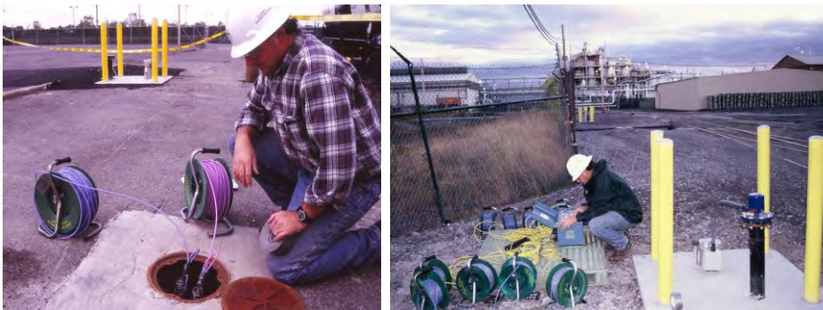
Figure 15.27 Hydrogeologist Andy Clark setting up a system for continuous monitoring of multiple monitoring wells at the startup of a pump-and-treat groundwater remediation at a site in New England. Cables from pressure transducers at the wells converge on the central datalogger.
