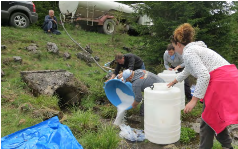
Figure 15.40 Dye tracing experiment with salt (NaCl) at one of the swallow holes in a karst aquifer of western Serbia. The water truck is used to dissolve large quantities of the tracer and chase it down the swallow hole. Courtesy of Zoran Stevanović.
