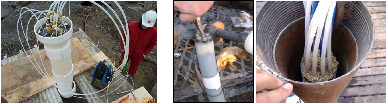
Figure 14.25 Examples of commercially available multi-level monitoring systems. Left photo : FLUTE, Flexible Liner Underground Technologies ( https://www.flut.com/ ). Two right photos : single-casing Multilevel Groundwater Monitoring System CMT by Solinst ( https://www.solinst.com/products/multilevel-systems-and-remediation/ ). All photos courtesy of Peter Thompson.
