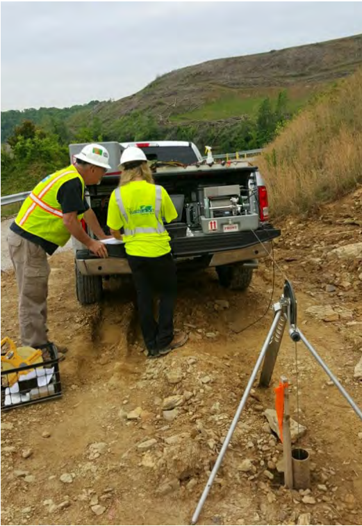
Figure 14.17 Geophysical borehole logging setup. Photo courtesy of Dawit Yifru.
