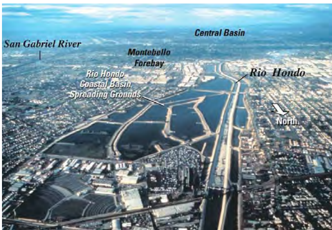
Figure 16.45 Rio Hondo Coastal Spreading Grounds in Montebello Forebay. From Anders and Schroeder, 2003. USGS, in public domain.
