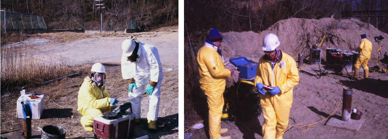
Figure 14.1 Use of personal protective equipment (PPE) during sampling of groundwater impacted by volatile organic compounds (left), and setup for an aquifer pumping test (right) by hydrogeologist Roger Pennifill and his crew of Ebasco Environmental, Inc. at Mattiace Petrochemical Superfund site, Glen Cove, New York.
