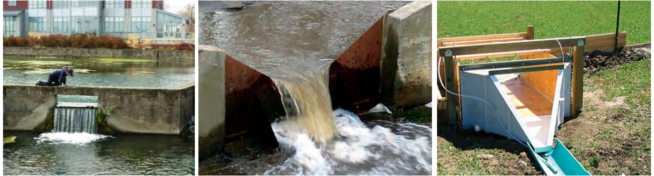
Figure 15.11 Left : Rectangular weir measuring outflow from a spring in Winchester, Virginia formerly utilized for public water supply. Middle : Sharp-crested 120 degrees V-notch weir. Right : Prefabricated H flume. Two right photographs courtesy of Don Meals, Tetra Tech, Inc., from NNPSMP, 2008; in public domain.
