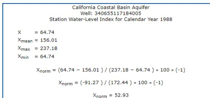
Figure 8 – Calculation of a normalized value for the Well: 340655117184005
