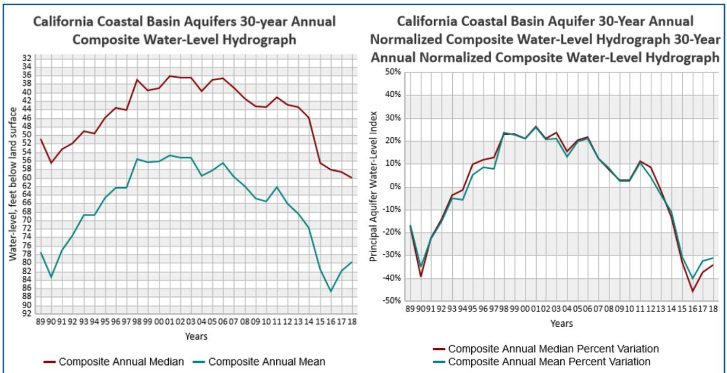
Figure 9 – Example of composite hydrograph (left) and example of normalized composite hydrograph (right). Source: USGS
