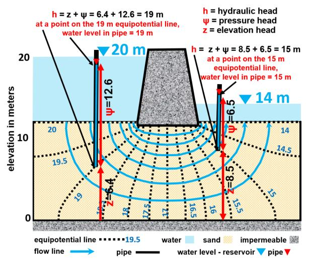
**Figure 3** - A cross-sectional view of a groundwater flow net under a dam from an upper reservoir to a lower reservoir. A flow net is comprised of two sets of lines that honor Darcy's Law and conserve mass. Equipotential lines connect points of equal hydraulic head (black dotted lines) and flow lines delineate paths of groundwater flow (blue solid arrows).
