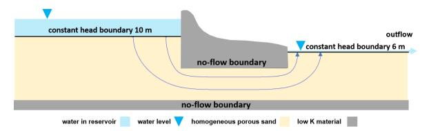
**Figure 7** - Step 4: Draw flow lines along paths where you envision groundwater flowing (blue arrows), ensuring they are perpendicular to equipotential lines on the boundaries. Do not be concerned about getting them right initially. Drawing flow nets is a trial-and-error process. As experience with flow nets grows, intuition improves and it becomes easier to place flow lines in nearly the right position on the first attempt.
