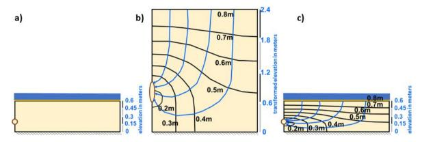
**Figure 18** - <u>Click to view Box 5</u><sup>1</sup> for the step-by-step process of drawing groundwater flow nets in anisotropic systems. Drawing an anisotropic flow net: a) Flow system geometry; b) Flow system transformed with flow net drawn for isotropic conditions; c) Flow system returned to untransformed geometry with flow net for anisotropic conditions.
