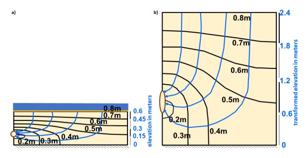
Figure Box 5-7 - The (b) isotropic flow net on the right is transformed back to the (a) anisotropic geometry on the left.
