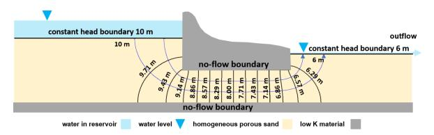
Figure 11 - Step 6: Calculate the equipotential line contour interval and label the equipotential lines. In this case the contour interval is ~0.29 meters.
