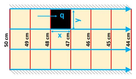
Figure Box 3-2 - Diagram for deriving equation to determine volumetric flow rate of a flow net per unit width into the diagram through one square of a flow net.
