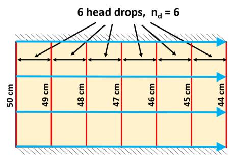
Figure Box 3-3 - Number of head drops in the example flow net.
