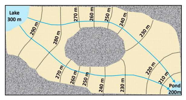
**Figure 4** - A plan view of flow in a confined aquifer penetrated by a deep lake and pond and laterally constrained by bedrock. The lake water elevation is 300 meters and the elevation of the pond surface is 200 meters. The top of the aquifer is 190 meters. Flow lines diverge on the upgradient side of the bedrock island in the middle of the aquifer and converge on the down gradient side.
