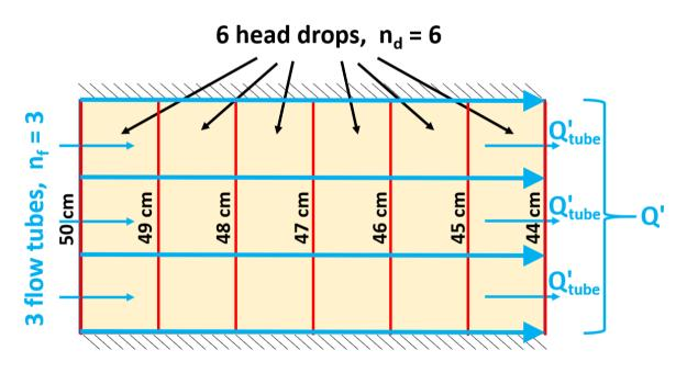
Figure Box 3-4 - Number of flow tubes and head drops in the example flow net.
