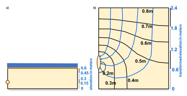
Figure Box 5-6 - An isotropic flow net is drawn in the transformed isotropic system (b) on the right.
