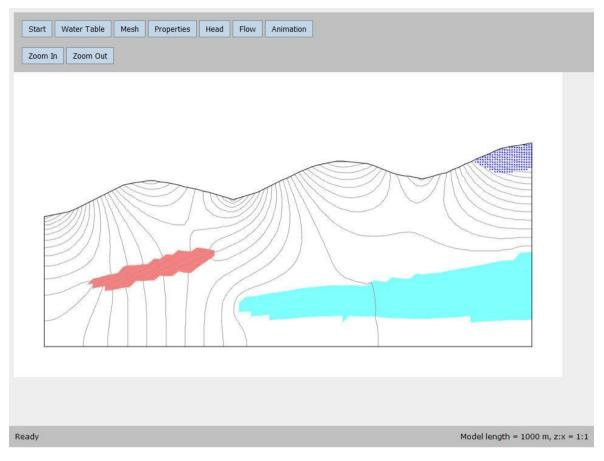
Figure Box 6-5 – Starting positions of a group of particles within the TopoDrive model.
