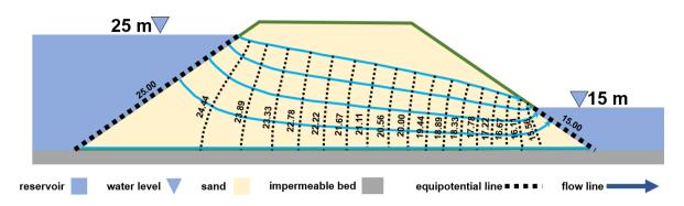
**Figure Box 4-5** - Draw equipotential lines for the unconfined flow net, ensuring that 1) their value is equal to the elevation of the water table where they meet the water table and to the elevation of the ground surface where they meet the seepage face, 2) that they meet flow lines at right angles, and 3) that the intersecting lines form curvilinear squares. This result was obtained after sketching and erasing until all of the criteria were met.
