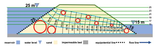
**Figure Box 4-4** - The shapes are curvilinear squares if circles fit approximately within them, but some flow nets may include partial flow tubes as shown here by the narrow flow tube at the bottom of the flow net. The flow net has 18 head drops and 4 flow tubes.
