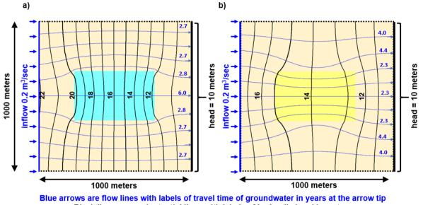
Black lines are equipotential lines with labels of hydraulic head in meters Dashed lines are no-flow boundaries
