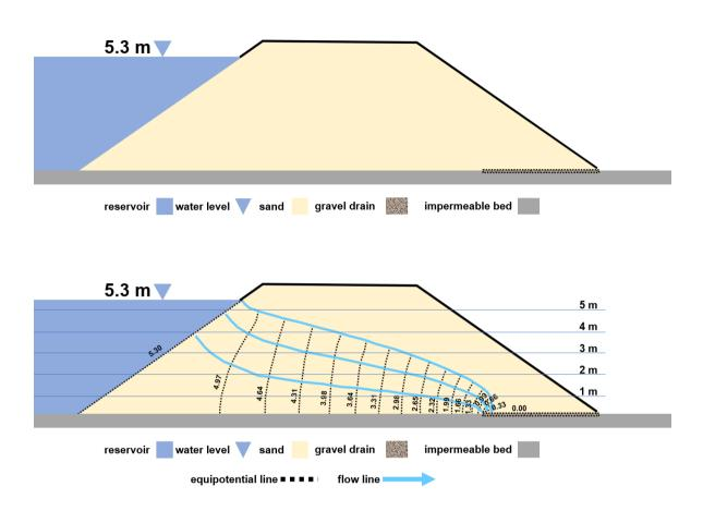
Contour interval = (5.3 m) / (16 head drops) = 0.33125 m
