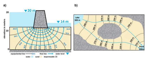
**Figure 2 -** Images of flow nets: a) groundwater moving in a vertical cross section under a dam; and, b) a plan view of groundwater flow from a lake to a pond surrounded by bedrock outcrops.
