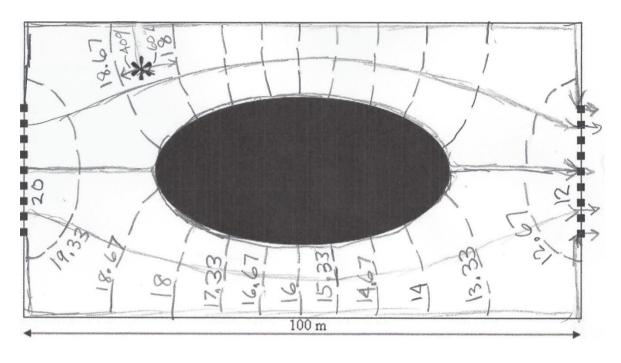
Contour interval =  $\frac{8m}{12 \text{ headdrops}} = 0.66$ Qtotal = KH  $\frac{nc}{nd}$  w =  $1 \times 10^{-3} \frac{m}{s} \frac{8m}{12} 10m = 0.26 \frac{m^3}{5}$ hydraulic head @  $\# \approx 18 + 0.6 \times 0.66 \approx 18.4 \text{ m}$ pressure head = hydraulic head-elevation = 18.4 m - 10 m = 8.4 m
