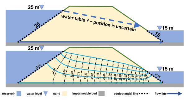
**Figure 13** – <u>Click here to go to Box 4</u> which describes the procedure for drawing a flow net with a water table boundary.
