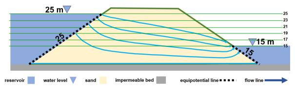
**Figure Box 4-3** - Add lines of equal elevation before sketching the equipotential lines, because the value of an equipotential line is equal to elevation where it intersects the water table and seepage face, so the elevation lines provide a guide for placing the equipotential lines.
