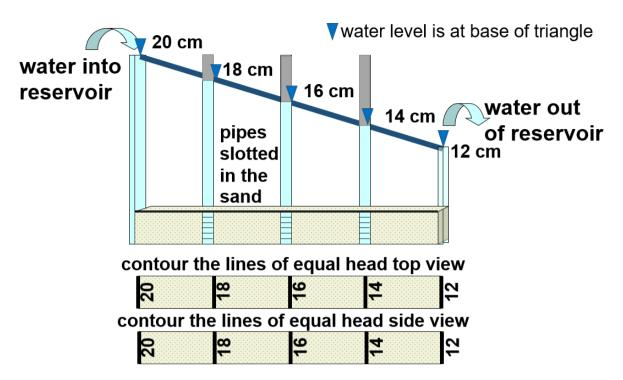
Figure Box 2-2 - According to Darcy's Law, hydraulic head declines linearly in a homogeneous material with a constant flow area.
