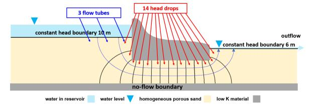
**Figure 10** - The appropriate number of head drops (spaces between equipotential lines) and flow tubes (spaces between flow lines) are determined by following the rules for drawing a flow net. This flow net has 14 head drops and 3 flow tubes.
