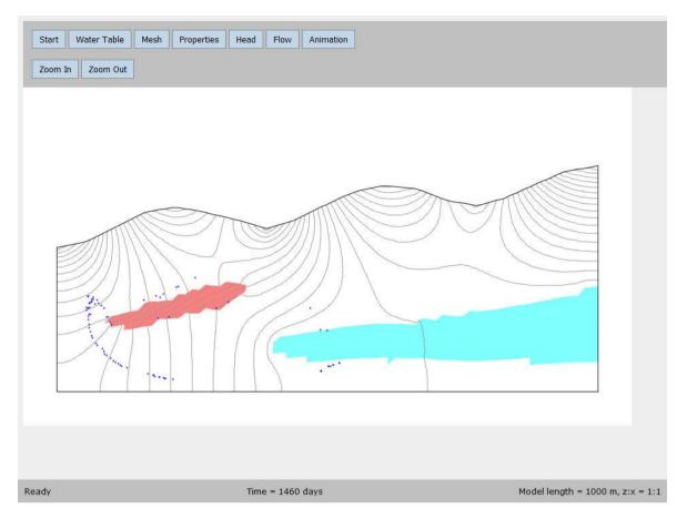
**Figure Box 6-7** - Particle positions after 1460 days (4 years). Many particles have exited the aquifer. A strand of particles is moving around the left side of the low hydraulic conductivity zone (pink region) and a few particles have moved into the low hydraulic conductivity zone.
