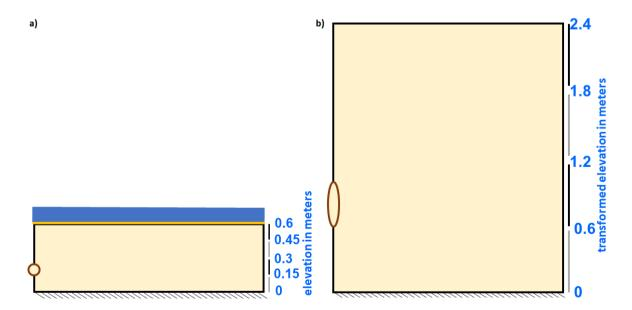
**Figure Box 5-5** - Geometric transformation of the (a) anisotropic system on the left to an (b) isotropic system on the right by transforming the vertical axis. The transformed geometry on the right is 4 times taller and as wide as the left one. The shape of the circular drain becomes an oval.
