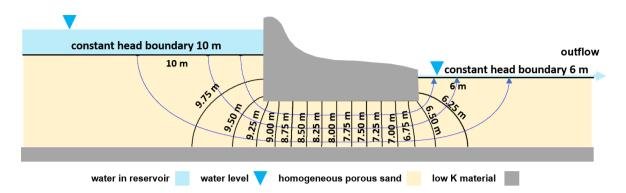
**Figure 12** - A flow net for the system illustrated in Figure 11 with a contour interval of 0.25 meters, requiring 3.43 flow tubes to achieve curvilinear squares and a valid ratio of the number of flow tubes to the number of head drops. Thus, the deepest flow tube is only ~40% of the width of the flow tubes that form curvilinear squares.
