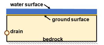
**Figure Box 5-4** Only a small portion of the field with parallel drains needs to be drawn to develop a flow net. A groundwater divide (no-flow boundary) occurs halfway between two adjacent drains. In addition, flow to the drain from the left is a mirror image of flow from the right. This symmetry enables us to consider the flow to the drain from only one side. The flow net developed for the above figure will repeat across the many drains of the field in alternating mirror images.
