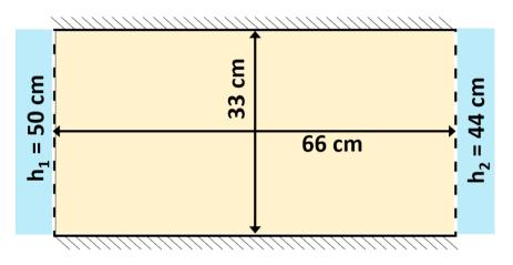
Figure Box 3-1 - A rectangular box filled with sand with constant head reservoirs on each side.
