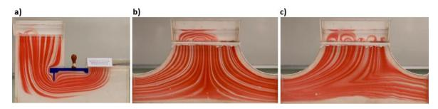
**Figure 14** - Hele-Shaw cells display flow paths for a) <u>Click to view</u> flow under a dam, b) <u>Click to view</u> flow of recharge from a ridge to a surrounding water body, c) <u>Click to view</u> flow of recharge from a ridge first to the lake on the right and then to the lake on the left. (- Videotaping of Hele-Shaw model simulations at the University of Hong Kong by J. Jiao and W.Z. Liang. Editing and voice over by Eileen Poeter.)
