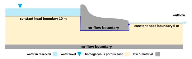
**Figure 6** - Step 1 - Draw the system to scale (no-flow boundaries are indicated by gray zones), Step 2 - Draw equipotential lines to coincide with head boundaries (black lines), Step 3 - Draw flow lines to coincide with no-flow boundaries (blue arrow following the no-flow boundary of the dam.
