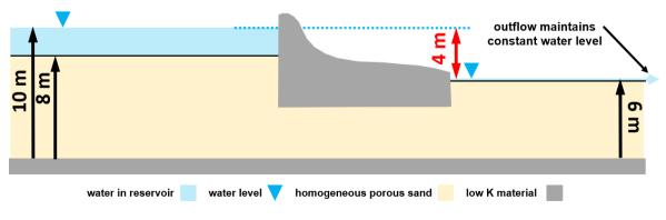
Figure 5 - A concrete dam keyed into soil.
