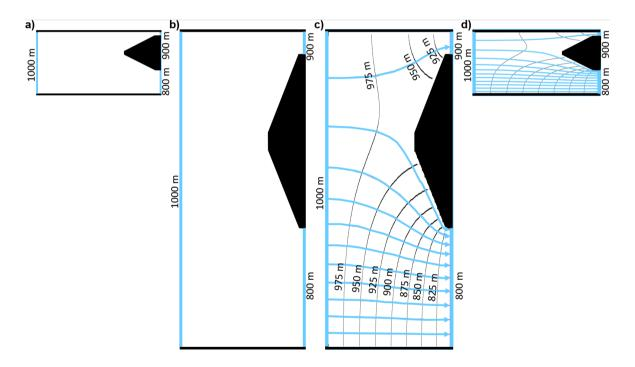
Contour interval = (200 m) / (8 head drops) = 25 m
