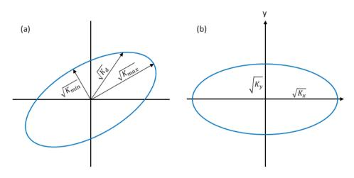
**Figure Box 5-1** - Hydraulic conductivity ellipse (a) in general orientation and (b) with major and minor axes aligned with the rectangular (x-y) coordinate system.
