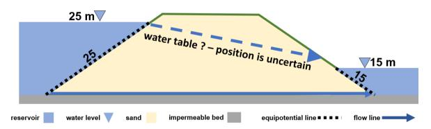
**Figure Box 4-1** - Step 1 - Draw the system to scale, Step 2 – Draw equipotential lines to coincide with head boundaries, Step 3 - Draw flow lines to coincide with no-flow boundaries.
