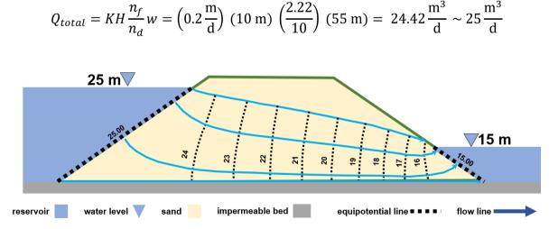
**Figure Box 4-6** - Some flow nets may include partial flow tubes as shown here by the narrow flow tube at the bottom of the flow net. The flow net has 10 head drops and 2.22 flow tubes.
